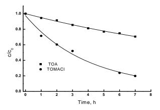
Fig. 1. Kinetics curves of perrhenate anions transport across PIM with TOA and TOMACl PIMs: 77 wt. % CTA, and 23 wt. % ion carrier; source phase: 0.0050 M ReO<sub>4</sub> in 0.10 M HNO<sub>3</sub>; receiving phase: 0.10 M NaOH
