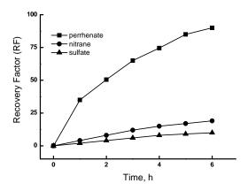
Fig. 3. Recovery factor (RF) vs. competitive transport of perrhenate, nitrate and sulfate on PIM with TOMACI. PIM: 1.0 M TOMACI, 0.8 cm<sup>3</sup> ONPOE / 1.0 g CTA; source phase:  $5 \cdot 10^{-4}$  M ReO<sub>4</sub><sup>-</sup> in 0.05 M HNO<sub>3</sub> and 0.05 M H<sub>2</sub>SO<sub>4</sub>; receiving phase: 0.10 M NaOH
