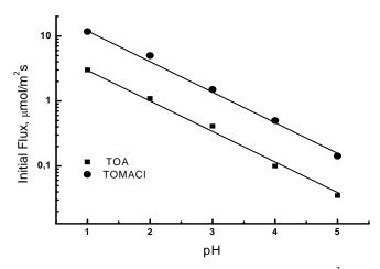
Fig. 2. Iinitial flux values vs. pH of the source phase. Membrane: 0.8 cm<sup>3</sup> ONPOE / 1.0 g CTA, 1.0 M carriers (TOA, TOMACI); source phase: 5·10<sup>-3</sup> M ReO<sub>4</sub>-, H(Na)NO<sub>3</sub> I=0.1 M
